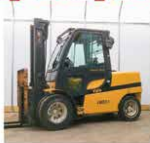
2019 Yale GDP120VXN Diesel, 12,000 lb cap, 2 stage, sideshift, fork positioning, 11,724 hrs $21,000 #255
