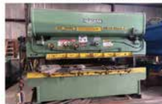
Niagara 60 Ton Press Brake Model 60-8-10 Mechanical Press Brake 10' Bed Total Bed Length Will Bend: 14Ga at 10', 12Ga at 8', 10Ga at 5' Price: $8,000.00
