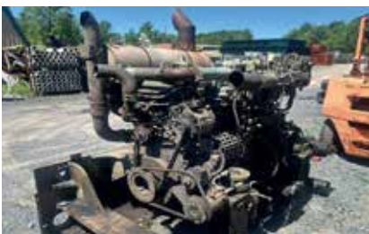
Izuzu Diesel Motor with Hydraulic Pump 6 Cylinder 349 HP 1800 RPM Previously powered a Hitachi 520 Excavator $7,500.00
