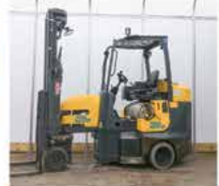
2019 Aisle Master 44SG LP , 4,400 lb cap, 3 stage, sideshift, fork positioning, 15,851 hrs $7,200
