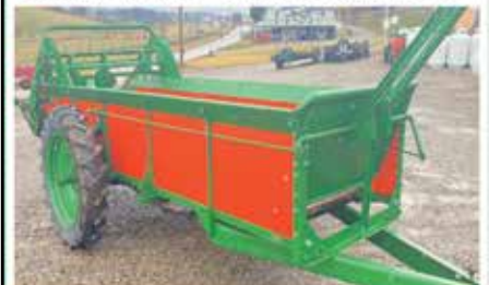
Rebuilt NI #17 – 85bu. Ground Drive
