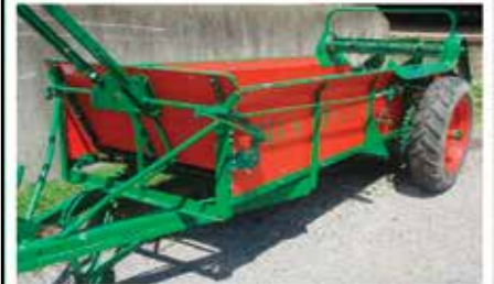
Rebuilt NI #12 – 85bu. Ground Drive
