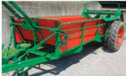
Rebuilt NI #12 – 85bu. Ground Drive
