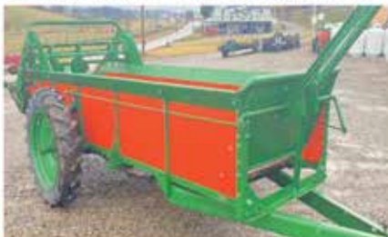
Rebuilt NI #17 – 85bu. Ground Drive
