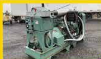
Detroit 671 100 KW Genset with Delco A.C. Y1-4634 Generator
