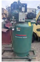
Champion Advantage Air Compressor , Champion Advantage Series Air Compressor, Model VR5-8: 80-Gallon Tank, 5 Horse Power Motor, 230Volt, 3 Phase, Maximum PSI 175 2 Available $2,800 Each
