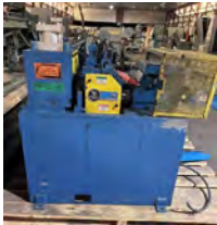
Coil Straightener Coe Press Equipment, LPRF-S206, Series 395, Maximum Material Width: 6". Maximum Material Width: 0.100 at 6" Wide, Thicker Narrow Stock Up to 0.125 at reduced width. Rated at 395 feet per minute. $9,500
