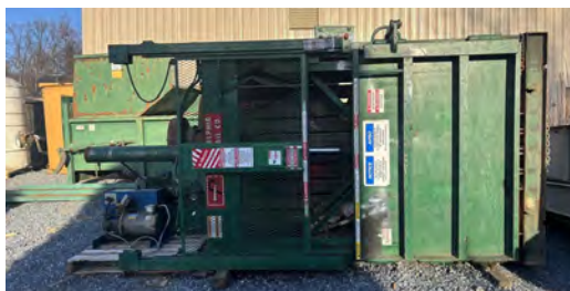
Philadelphia Cardboard Baler, Philadelphia Tramrail Vertical, Hydraulic, Cardboard Baler 30"x60" Chamber, Vertical hydraulic cardboard baler / trash compactor, Hydraulic compression for consistent, dense bales $5,700
