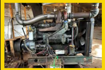
Detroit 671 Power Unit
