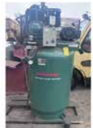
Champion Advantage Air Compressor. Champion Advantage Series Air Compressor, Model VR5-8: 80-Gallon Tank, 5 Horse Power Motor, 230Volt, 3 Phase, Maximum PSI 175.2 Available $2,800 Each
