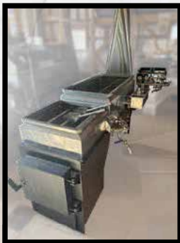
Evaporator Dropped Flue Model
