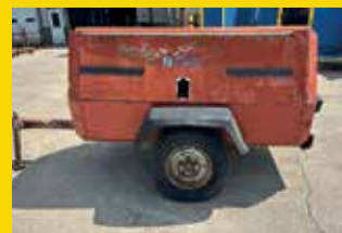
Ingersoll-Rand Portable Air Compressor
