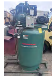
Champion Advantage Air Compressor, Champion Advantage Series Air Compressor, Model VR5-8: 80-Gallon Tank, 5 Horse Power Motor, 230Volt, 3 Phase, Maximum PSI 175 2 Available $2,800 Each
