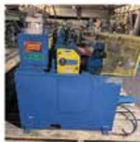
Coil Straightener Coe Press Equipment, LPRF-5206, Series 395, Maximum Material Width: 6". Maximum Material Width: 0.100 at 6" Wide, Thicker Narrow Stock Up to 0.125 at reduced width. Rated at 395 feet per minute. $9,500
