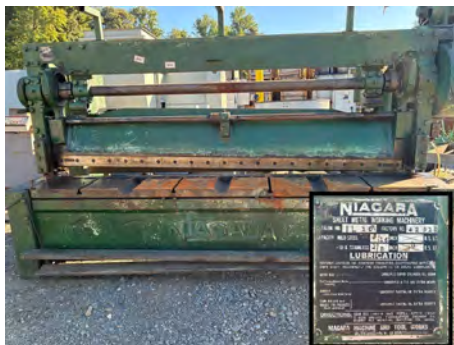
Niagara Machine & Tool Works IL-10 Power Squaring Shear Shear Capacity Mild Steel 3/16" / Stainless 1/8" Price: $4,000.00
