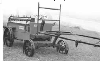
EZ-30 30 bushel, 3-beater design for pen packed manure
