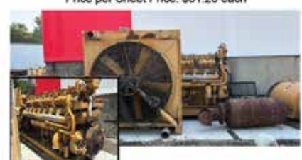
Kato Engineering 1030 AC generator / 16 Cylinder Cat D399 Diesel Motor Generator Set Generator Capacity: 1030 kW continuous duty. Voltage: 346/600V or 480V, 3-phase. Cat D299 Diesel Motor: 1,250 HP at 1,200 RPM Price: $35,000.00 (1 Available)
