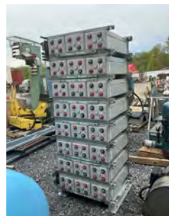
Absolyte GP VRLA AGM Battery 8 Bank System Great for use with Solar Power System Each Bank is: 6 Volt, 1,000 Nominal Amp-Hour Capacity (Over 8 Hrs) $2,500.00
