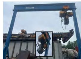
Gorbel Gantry Crane 3 Ton Capacity 14' High x 12' Width x 7' Base Harrington 3 Ton Capacity Electric Hoist $5,500.00
