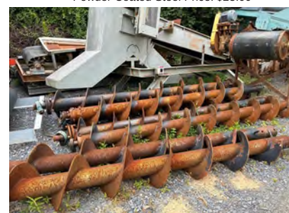
12-1/2' and 30' (Total Lengths) 12-1/2' Flight- Flight Diameter 16", Shaft Diameter 6-3/4", Flight Thickness 3/4" 30' Long Flight- Flight Diameter 18", Shaft Diameter 6-1/2", Flight Thickness 3/4" Price: 12-1/2' $500.00 each 30' $1,000.00 each
