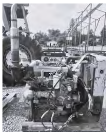
Cat 3304 , 115 HP, Radiator Thru Flywheel, 3000 Hrs, $4,500
