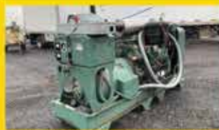
Detroit 671 100 KW Genset with Delco A.C. Y1-4634 Generator
