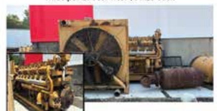
Kato Engineering 1030 AC generator / 16 Cylinder Cat D399 Diesel Motor Generator Set Generator Capacity: 1030 kW continuous duty. Voltage: 348/600V or 480V, 3-phase. Cat D299 Diesel Motor: 1,250 HP at 1,200 RPM Price: $35,000.00 (1 Available)
