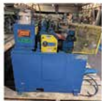
Coil Straightener Coe Press Equipment, LPRF-S206, Series 395, Maximum Material Width: 6". Maximum Material Width: 0.100 at 6" Wide, Thicker Narrow Stock Up to 0.125 at reduced width. Rated at 395 feet per minute. $9,500
