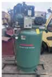
Champion Advantage Air Compressor, Champion Advantage Series Air Compressor, Model VR5-B: 80-Gallon Tank, 5 Horse Power Motor, 230Volt, 3 Phase, Maximum PSI 175 2. Available $2,800 Each
