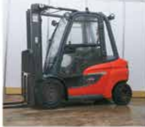
2020 Linde H35D Diesel, 7000 lb cap, 2 stage, sideshift, 1,480 hrs $34,100
