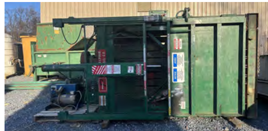
Philadelphia Cardboard Baler, Philadelphia Tramrail Vertical, Hydraulic, Cardboard Baler 30"x60" Chamber, Vertical hydraulic cardboard baler / trash compactor, Hydraulic compression for consistent, dense bales $5,700
