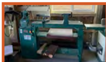
Grizzly G1495 - heavy duty wood lathe w/ end plate attachment, 3/4 HP, 110V
