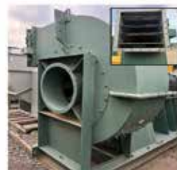
New York Blower Company Series 45 General Industrial Blower Intake Flange 30" Exhaust Flange 25"x29" 1 EA 125HP Motor 10,000ACFM Cost: $12,000.00 1 EA 200HP Motor 20,000ACFM Cost: $18,000.00
