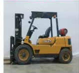
Cat GP40 LP , 8,000 lb cap, 2 stage, sideshift, 8,215 hrs antifreeze leak, no parking brake, $6,000
