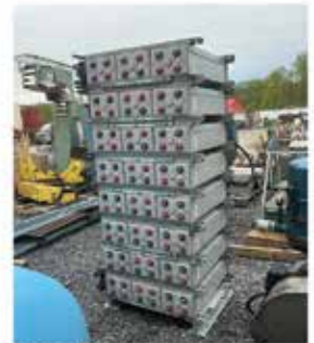
Absolyte GP VRLA AGM Battery 8 Bank System Great for use with Solar Power System Each Bank is: 6 Volt, 1,000 Nominal Amp-Hour Capacity (Over 8 Hrs) $2,500.00
