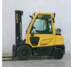
2021 Hyster H60FT LP , 6,000 lb cap, 3 stage, sideload, fork positioning, 1,269 hrs $21,500
