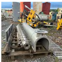
Stainless Steel Industrial Screw Auger Conveyor (Less Motor) Flight 10'-1/2" L, 12" Diameter, Shaft 3" Housing 13"W, 14"D 11' Long Price: $5,000.00
