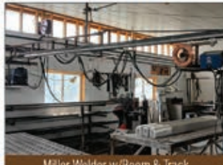
Miller Welder w/Boom &amp; Track
