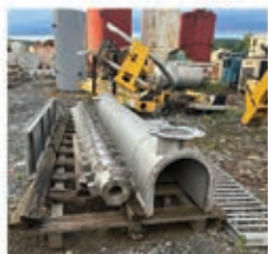
Stainless Steel Industrial Screw Auger Conveyor (Less Motor) Flight 10'-1/2" L, 12" Diameter, Shaft 3" Housing 13"W, 14"D 11' Long Price: $5,000.00
