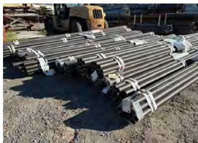
3-3/4" DOM Tubing (Just off the truck) 3.25" OD x 2.624 ID (.313 Wall) Steel Tube 4,900' Available Priced by Pound Price: $0.50 Per Pound
