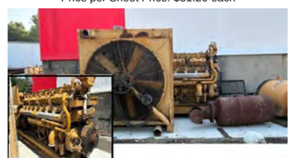
Kato Engineering 1030 AC generator / 16 Cylinder Cat D399 Diesel Motor Generator Set Generator Capacity: 1030 kW continuous duty. Voltage: 346/600V or 480V, 3-phase. Cat D299 Diesel Motor: 1,250 HP at 1,200 RPM Price: $35,000.00 (1 Available)
