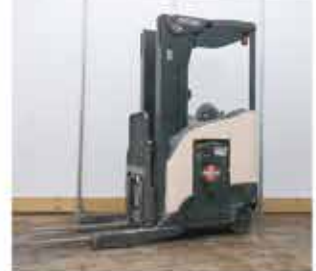
2019 Crown RR5725-35 EL , 36V, 3,500 lb cap, 3 stage, sideshift, 9,783 hrs $5,700
