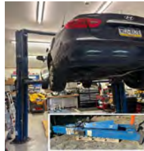
Rotary Car Lift Model SPOA7-200 7,000 Pound Dual Post Lift With 74" Lift height Price: $1,800.00
