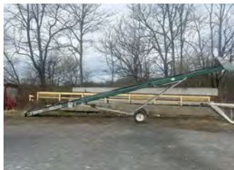
Portable Doyle Conveyor 480 Volts 24" Wide X 40' Long Max Height 25' Belt and some rollers need replaced $4,500.00
