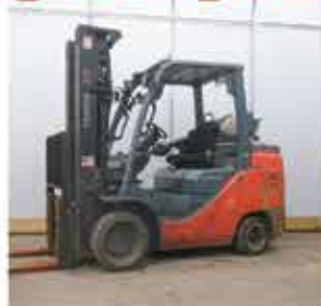
2016 Toyota 8FGC45U LP, 10,000 lb cap, 3 stage, sideload, fork positioning, 8,658 hrs $13,200
