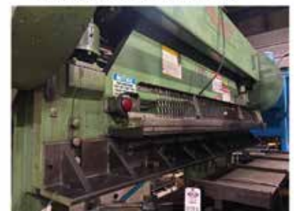
Cyril Bath Model C Press Brake Heavy duty industrial Mechanical Press Brake, 150 Ton Capacity with a 10' Bed Great for precision Sheet Metal Bending of stainless steel, mild steel, and aluminum parts. Price: $11,999.99
