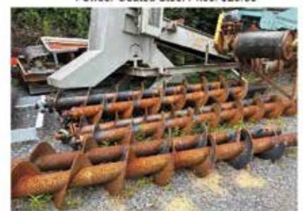
12-1/2' and 30' (Total Lengths) 12-1/2' Flight-Flight Diameter 16", Shaft Diameter 6-1/2", Flight Thickness 1/2" 30' Long Flight-Flight Diameter 18", Shaft Diameter 6-1/2", Flight Thickness 1/2" Price: 12-1/2' $500.00 each 30' $1,000.00 each
