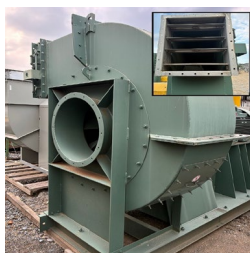
New York Blower Company Series 45 General Industrial Blower Intake Flange 30" Exhaust Flange 25"x29" 1 EA 125HP Motor 10,000ACFM Cost: $12,000.00 1 EA 200HP Motor 20,000ACFM Cost: $18,000.00
