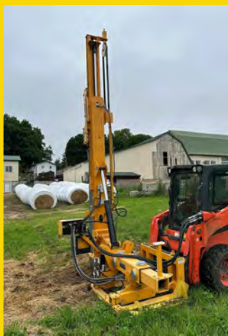
2022 Rhino Solar Pro Pile Driver Hillpoint, WI
