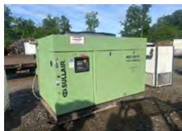
Sullair Air Compressor Model VCC-200S Mfg Date 2013 460 Volt 200HP 175 PSI Full Load 720 ACFM $12,000.00
