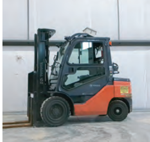
2020 Toyota 8FGU32 LP , 6,500 lb cap, 3 stage, sideshift, fork positioning, 7,194 hrs $22,500
