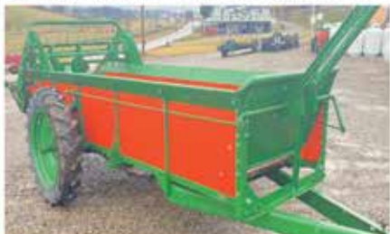
Rebuilt NI #17 – 85bu. Ground Drive
