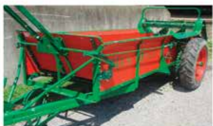
Rebuilt NI #12 – 85bu. Ground Drive
