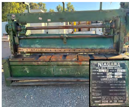
Niagara Machine & Tool Works IL-10 Power Squaring Shear Shear Capacity Mild Steel 3/16" / Stainless 1/8 Price: $4,000.00
