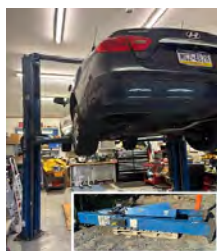
Rotary Car Lift Model SPOA7-200 7,000 Pound Dual Post Lift With 74" Lift height Price: $1,800.00
