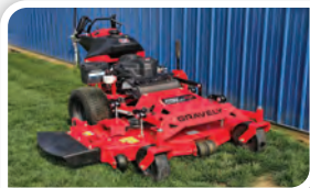
52" Gravely Pro-Walk Heavy duty commercial machine with 18.5 HP Kawasaki engine. Single point deck lift with 15 cutting positions. $9500
